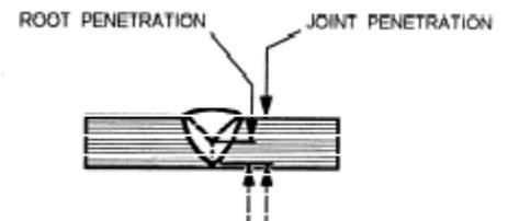
➤ In some cases, root penetration and joint penetration, can refer to the same dimension.
